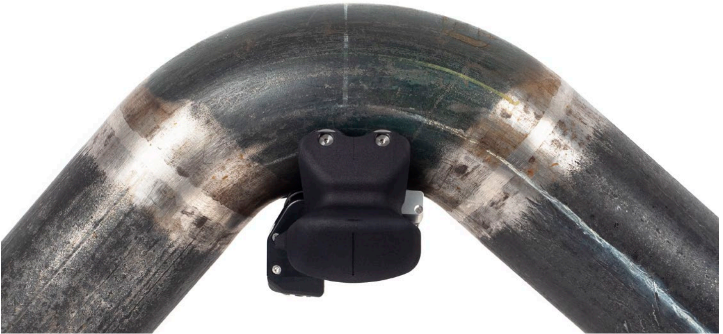
The FlexoFORM scanner inspecting the intrados of a 4.5 in. OD pipe elbow.
