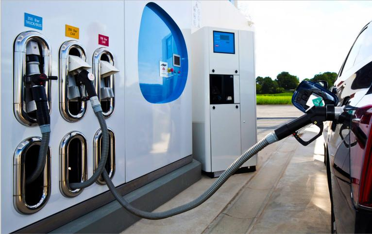
Fuelling process for an electric fuel cell vehicle using the WEH® fuelling nozzle TK17 H<sub>2</sub> 70 MPa
