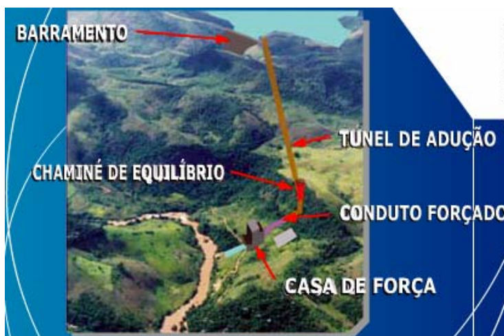
Figure 1 – Picada power plant location and physical configuration Source: www.usinapicada.com.br
